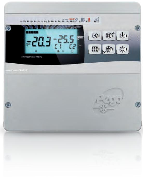
Electronic control for double system management with the possibility of inserting an environment secondary probe to ensure the proper operation of the system in case of environment main probe failure. Can manage up to two compressors and two evaporators, operating in call rotation mode (for even utilisation) or with a double set-point.
